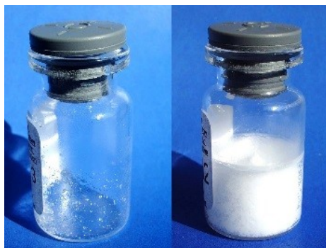
Figure 4: Freeze Dried Cakes with Collapsed (L) and Good (R) Structure
