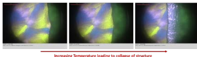
Figure 2: Images of sucrose under vacuum & upon heating from FDM
